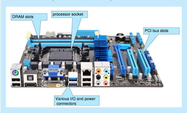
This board is a fully-functioning computer, once its slots are populated. It consists of a processor socket containing a CPU, DRAM sockets, PCIe bus slots, and I/O connectors of various types. Even the lowest-cost general-purpose CPU contains multiple cores. Some motherboards contain multiple processor sockets. More advanced computers allow more than one system board, creating NUMA systems.
